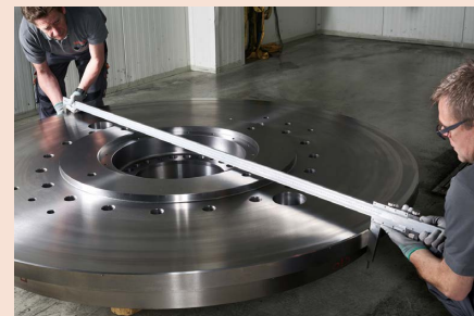
Radiused jaws for accurate ID measurement
